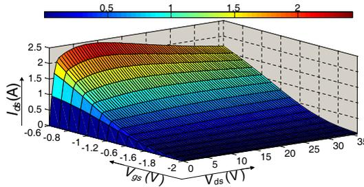
Figure 3. The solid database of  $I_{ds}$  established in Matlab.
