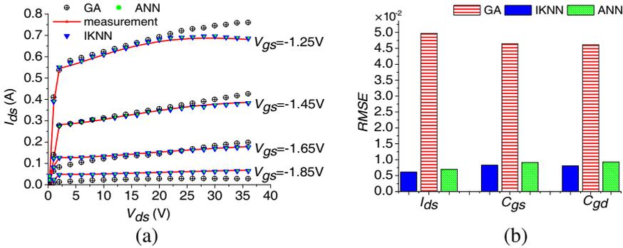
**Figure 6.** (a) The comparison of  $I_{ds}$  based on IKNN predicted results, GA predicted results, and measured results. (b) The comparisons of RMSE between IKNN, GA and ANN models.
