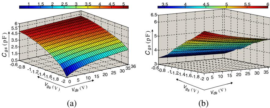
Figure 4. The solid databases of (a)  $C_{gs}$  and (b)  $C_{gd}$  established in Matlab.
