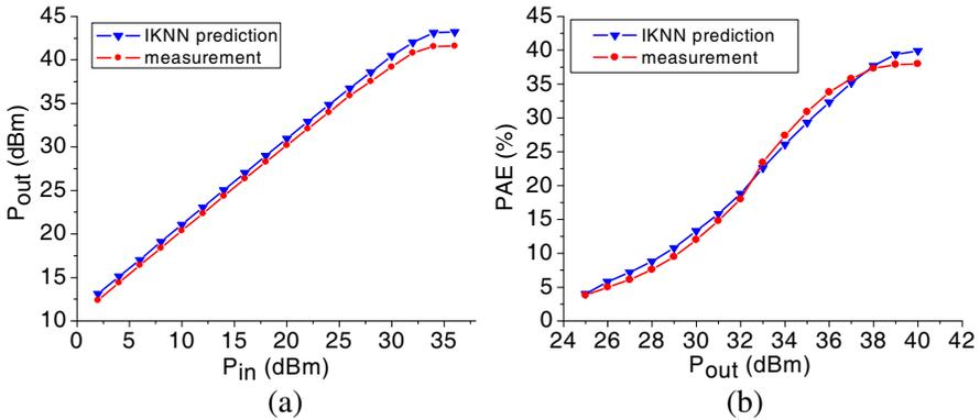
**Figure 8.** (a) the output power versus input power simulated by IKNN based model and measured result ( $f = 3$  GHz). (b) The power added efficiency ( $PAE$ ) simulated by IKNN based model and measured result ( $f = 3$  GHz).
