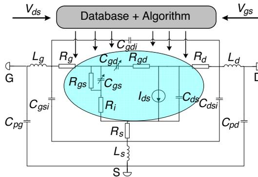
**Figure 1.** The large signal equivalent circuit for GaN HEMT device.
