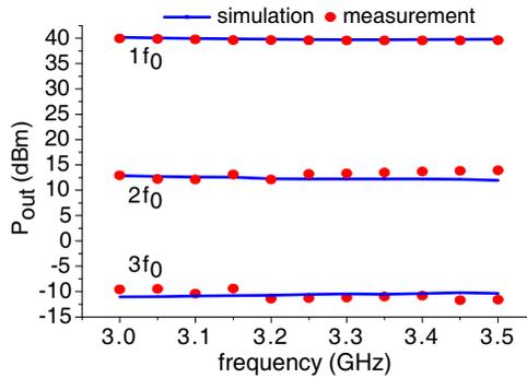
**Figure 7.** The Output power based on IKNN model and measurements ( $P_{in} = 30$  dBm).
