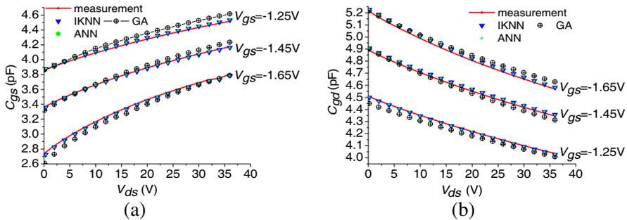
**Figure 5.** (a) The comparisons of  $C_{gs}$  based on IKNN predicted results, GA predicted results, and measured results. (b) The comparisons of  $C_{gd}$  based on IKNN predicted results, GA predicted results and measured results.
