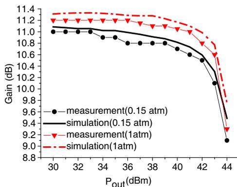
**Figure 6.** The comparisons of simulating gains and measurements under the two AP conditions ( $f = 3$  GHz).
