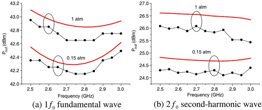
**Figure 7.** The compared results of simulating harmonic performances and measurements under the two AP conditions. ( $P_{in} = 32$  dBm).
