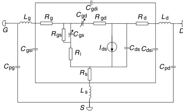
**Figure 2.** Typical equivalent circuit model of GaN HEMT device.
