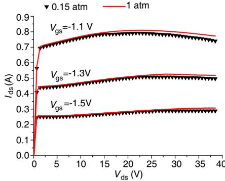
**Figure 1.** The comparisons of measured  $I_{ds}$  between two AP conditions.
