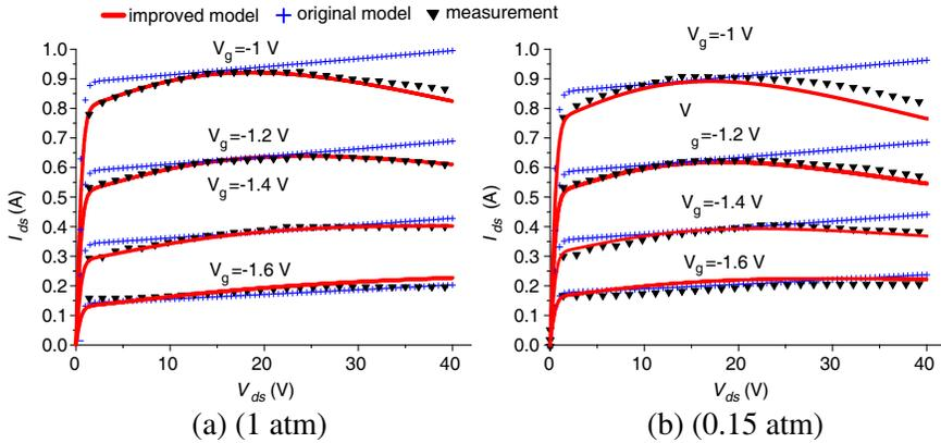
**Figure 4.** The compared results of simulated and measured  $I_{ds}$  under the two AP conditions. (a) is 1 atm, (b) is 0.15 atm.
