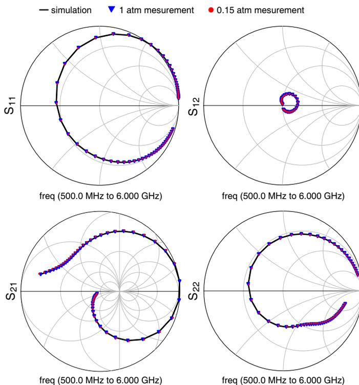
**Figure 5.** Simulated small  $S$ -parameters and measurements under the two AP conditions (0.5–6 GHz).
