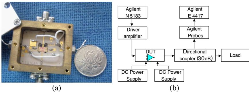
**Figure 3.** (a) The power amplifier for validation. (b) Measurement setup for power amplifier.
